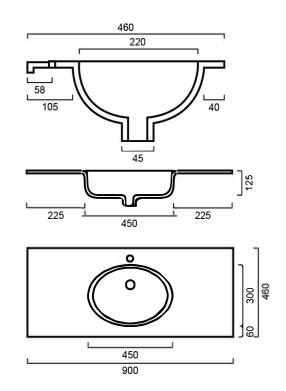
DIMENSIONS 900mm length x 460mm width x 125mm depth
